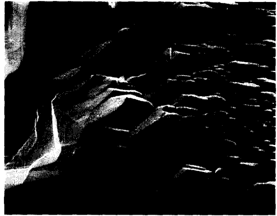
Fig. 2. Scanning electron micrograph of a (100) magnetite slice after 30 min non-ultrasonic etch in 12 M HCl (aq) , edge region.
